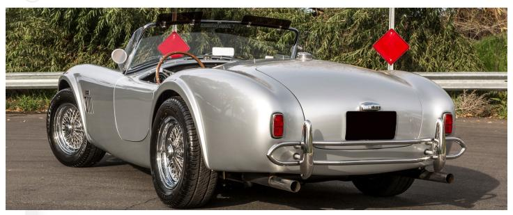
Slabside's feature straight cut fenders, where as the FIA features rolled fenders. FIA exhaust optional.
