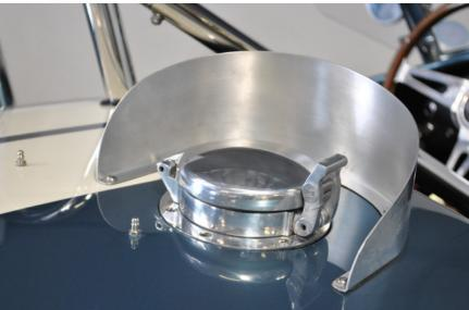
Optional Fuel cap diffusers can be fitted to FIA model cars.
