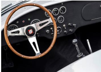
Slabside cars have the traditional roadster layout. FIA cars have two dash options, FIA and USSRC Spec.Aluminum interior is standard for FIA cars, where as carpeted surfaces are standard for Slabside cars. Glove boxes are standard for Slabside cars. (Leather seating shown optional)
