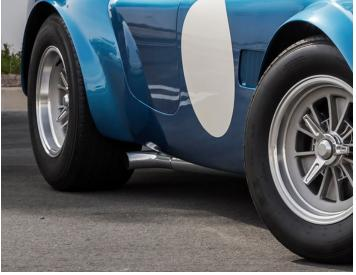
Sladside cars have under car exhaust, where as FIA cars have side exhaust standard.
